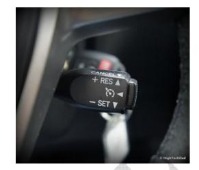
The driver can set the cruise control with the cruise switches, which usually consist of ON, OFF, RESUME, SET/ACCEL and COAST. These are commonly located on the steering wheel or on the windshield wiper or turn signal stalk. The SET/ACCEL knob sets the speed of the car. One tap will accelerate it by 1 mph, two by 2 mph and so on. Tapping the knob in the opposite direction will decelerate the vehicle. As a safety feature, the cruise control system will disengage as soon as we hit the brake pedal.
