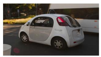
This car has a total of eight sensors. The most noticeable one is the rotating roof-top LiDAR – a camera that uses an array of 32 or 64 lasers to measure the distance to objects in order to build up a 3D map at a range of 200m, enabling the car to analyze potential hazards.
